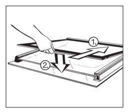
Fit the middle pane with the matt printed surface facing downwards.
